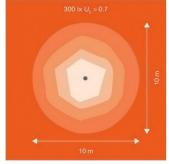
Floodlight Max 900W SYM 30 simplified isolux diagram
