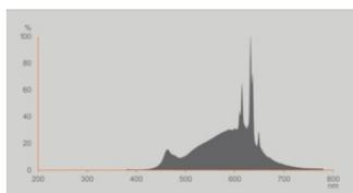
EPREL Data Spectral Diagram LEDr
