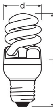
D TWIST 12 W/2700K 220...240 V E27, D TWIST 12 W/4000K 220...240 V E27, D TWIST 12 W/6500K 220...240 V E27
