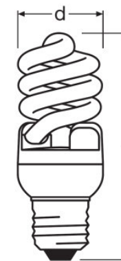
DTW 15 W/2700K 220...240 V E27, DTW 15 W/4000K 220...240 V E27, DTW 15 W/6500K 220...240 V E27
