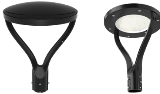
LPT100MWTC 100/75/50/30W Diameter Ø420mm x H 551mm Flex fit for 73-78mm pole
