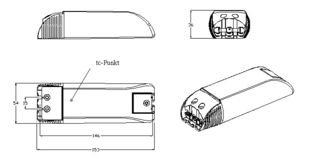
Max. allowed temperature at test point in normal operation:  $t_C \leq 80~{\rm °C}$
