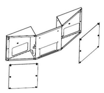
2. Next, attach the SBS mounting plate to the pedestal with (10) M5 provided screws.
