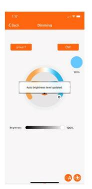
The lights will read the current light level from sensors and also record the current color temperature and save them as the auto light level.
