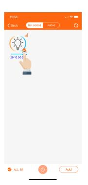
Click the **checkbox** on the bottom right corner of the light to add/remove this light.
