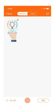
APP will scan and list all the nearby lights that can be added to the zone. To locate any **light** you can turn on/off by pressing the icon as above.
