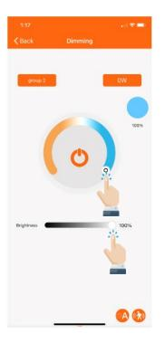
Use the wheel to control the CCT and slider to control brightness.
