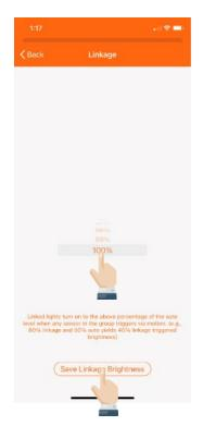
Set the linkage brightness level on the dimming control. Click "Save Linkage Brightness" button to save the setting.
