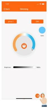
If there are lights with sensors in this group, then you may set the sensors parameter by clicking the **sensor icon** on the bottom right corner.
